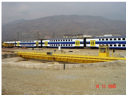
140 t x 27.5 m – sini davvar (Metro Tehran)
